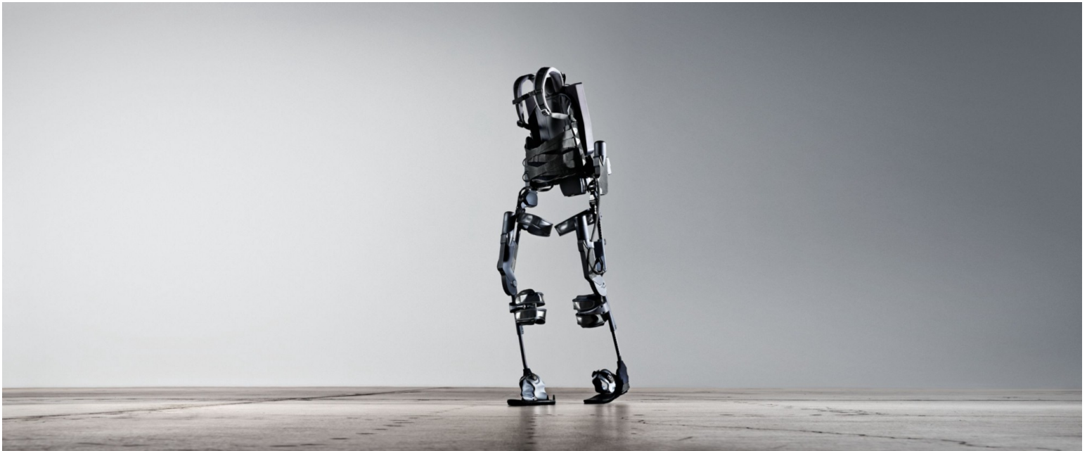
The “Ekso,” a commercially available wearable exoskeleton, designed to encase the length of the body in a harness for support and augmented strength. It has enabled some wheelchair users to walk upright.
